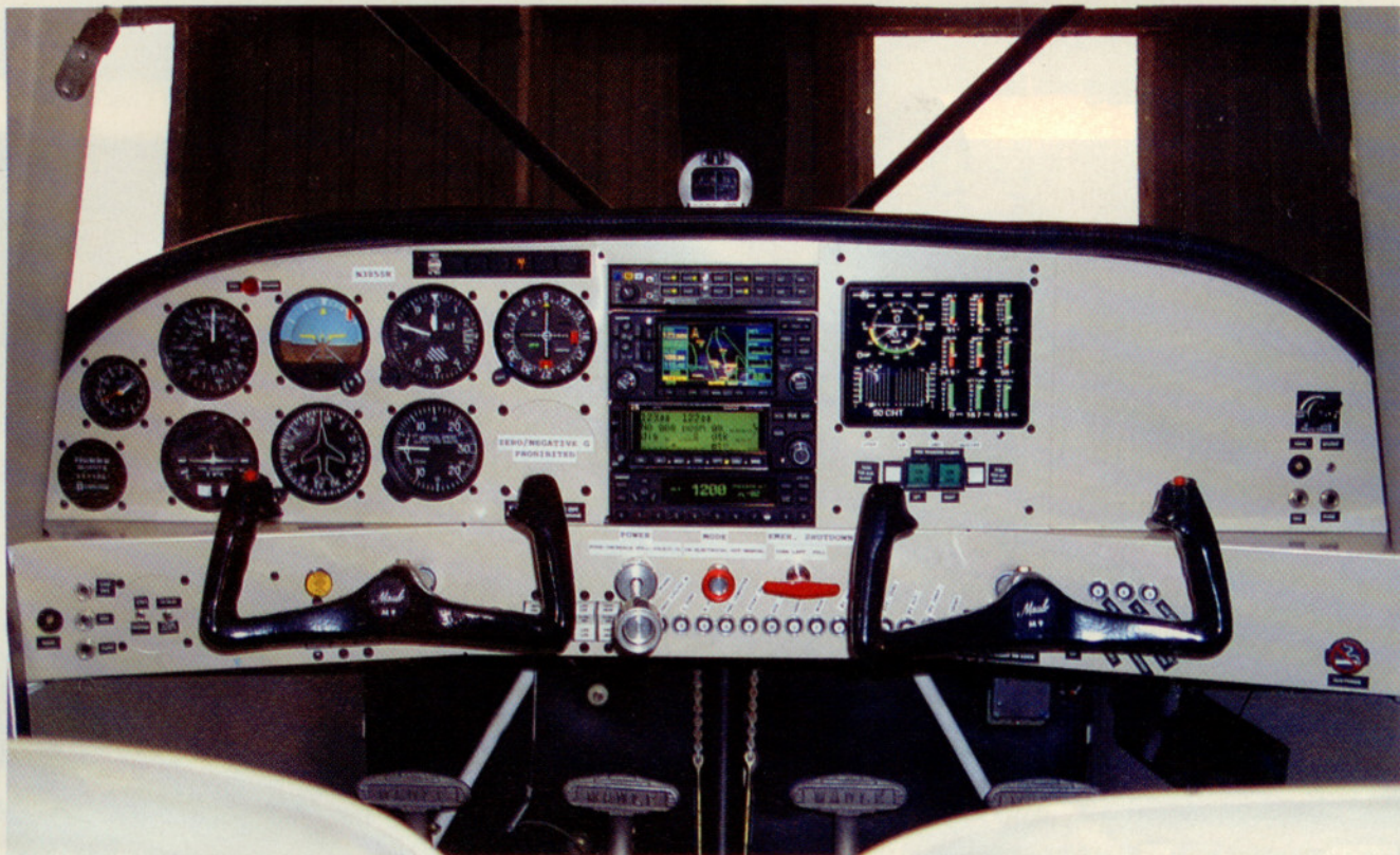
Only three levers are needed to control the engine, and of those, only one, the power lever, will see much use. The other two are used in the event of computer failure or emergencies. Maule installed a JPI EDM 930 engine instrument display to record engine performance during testing. The aircraft has two batteries, two alternators, and electric attitude and heading indicators.
